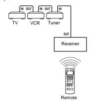
The remote sensor on this unit receives remote codes the same way as the remote sensor on the CTRL S IN component. This is useful if you place the other component away from this unit.
